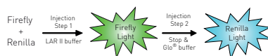
Fig. 2: Dual Luciferase Reaction - Luciferase Assay Reagent II (LAR II) is injected in the first step and the Firefly reaction is started. Stop and Glo® buffer is injected in the second step, which quenches the Firefly reaction and initiates the Renilla reaction.
