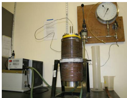
Fig. 1: The 3 litre pressure vessel used in this study.
