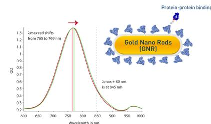
**Fig. 1:** Gold Nano Rods have an LSPR signal that can be detected with full spectral absorbance. The LSPR peak red-shifts upon ligand binding to the GNR surface, which is instantly captured by the spectrometer.
