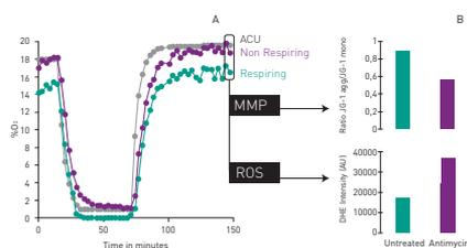
**Fig. 4:** Multiparametric analysis of Cor4U cells during *in vitro* ischemia-reperfusion validating multiplexed measurement of MitoXpress Intra and JC-1/DHE. Cell oxygenation traces describe depth and duration of Cor.4U ischemia-reperfusion (A) with parallel monitoring of MMP and ROS (B).
