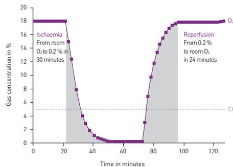
**Fig. 1:** Example of ischemia-reperfusion atmospheric conditions in the CLARIOstar microplate reader with ACU. O<sub>2</sub> and CO<sub>2</sub> levels were regulated as defined in the reader software.
