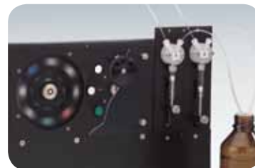
...reagent injection and fast filter switching
