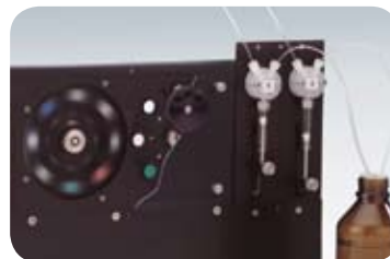
...reagent injection and fast filter switching
