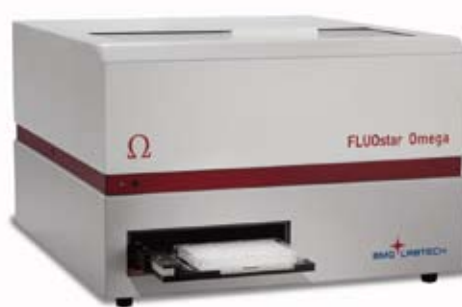
Fig. 1: BMG LABTECH's FLUOstar Omega multidetection microplate reader
